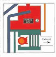
Generator, leaving a concentrated solution that is returned to the Heat Exchangers.
