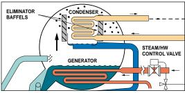
The refrigerant vapor migrates through mist eliminators to the condenser tube bundle. The refrigerant vapor condenses on the tubes. The heat is removed by the cooling water which moves through the inside of the tubes. As the refrigerant condenses, it collects in a trough at the bottom of the condenser.
