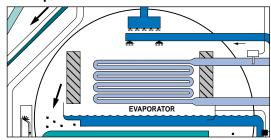
The refrigerant liquid moves from the condenser in the upper shell down to the evaporator in the lower shell and is sprayed over the evaporator tube bundle. Due to extreme vacuum in the lower shell (6mm Hg (0.8kPa) absolute pressure), the refrigerant liquid boils at 39°F (3.9°C), creating the refrigerant effect. (The vacuum is created by hygroscopic action - the strong affinity lithium bromide has for water - in the absorber directly below.)
