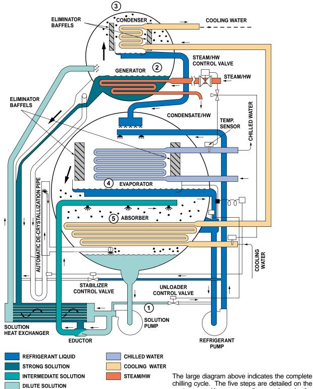
chilling cycle. The five steps are detailed on the next page with corresponding numbers in the diagram to show where each step is taking place. The cycle is continuous: however, for the sake of clarity and simplicity, it is divided into five steps.
