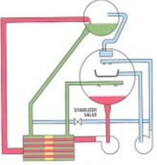
Unit senses a blockage due to crystalization, and opens the stabilzer valve.
