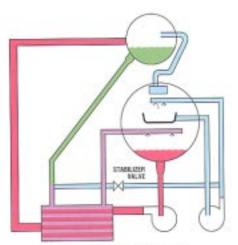
Diluted solution quickly dissolves crystals, leaving unit running smoothly.
