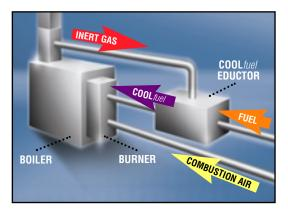
Inert gas is induced via existing fuel pressure into the **COOL***fuel* eductor to dilute and cool the flame, thereby reducing emissions. Additional NOx reduction can be achieved by injecting steam into the eductor to further dilute the fuel and induce larger amounts of inert gas.
