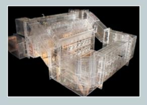
combustion air system, corrects distribution, eliminates unwanted swirl and improves flame stability. **COOL***flow* can also assist in the design of staged combustion air systems, such as over fire air or FGR, to maximize emissions reduction while reducing system pressure drop and horsepower requirements.
