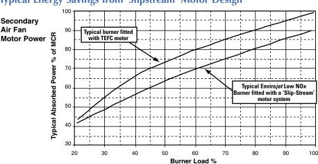
The above comparison is based on generic motor efficiencies and does not take into account the use of high efficiency motors
