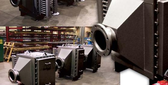
The Rock River Water Reclamation District covers nearly 88 square miles of Winnebago County and serves over 250,000 people. During the treatment process, the anaerobic digester speeds up the breakdown of solid waste which produces methane gas. This gas is used as a fuel to operate an engine generator. The heat is recovered from the generator by Cain heat recovery units and is used to heat the digester. The facility saves the district approximately \$40,000 each month in electricity.
