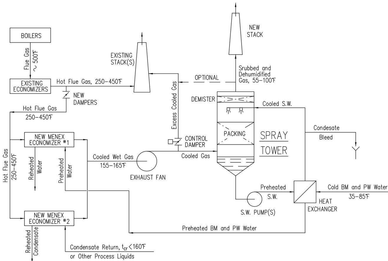
FIGURE 2. MENEX TWO-STAGE HEAT RECOVERY (TSHR) SYSTEM.
