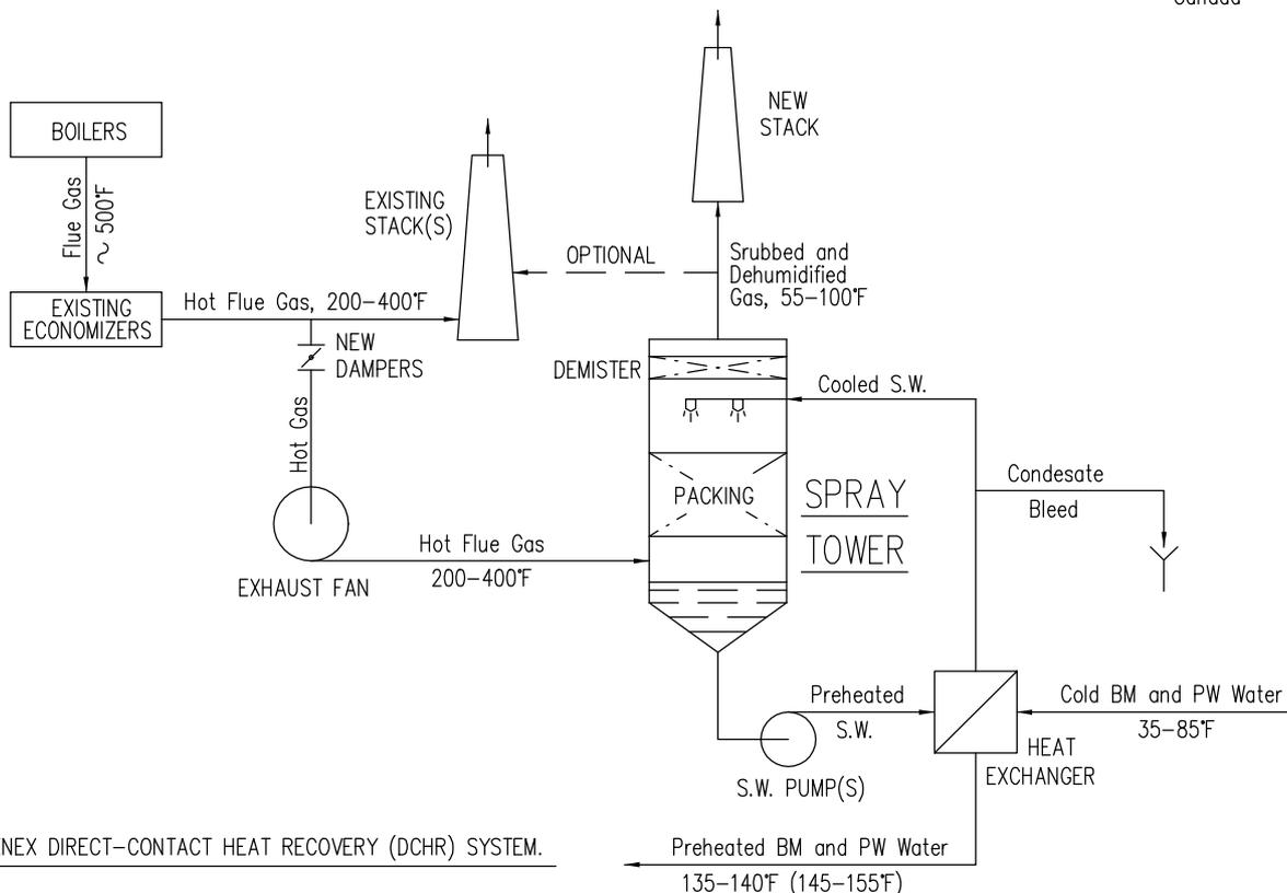
FIGURE 1. MENEX DIRECT-CONTACT HEAT RECOVERY (DCHR) SYSTEM.
